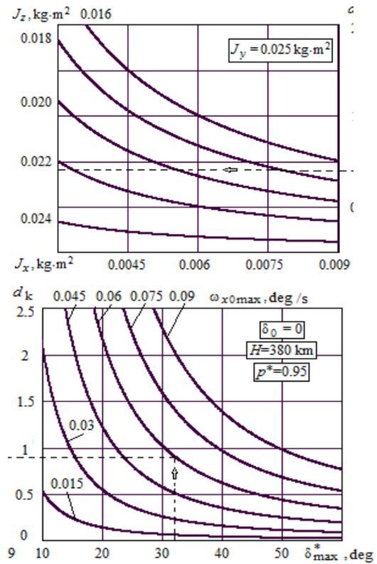
Fig. 1. Nomogram for selecting the design parameter of a nanosatellite.
