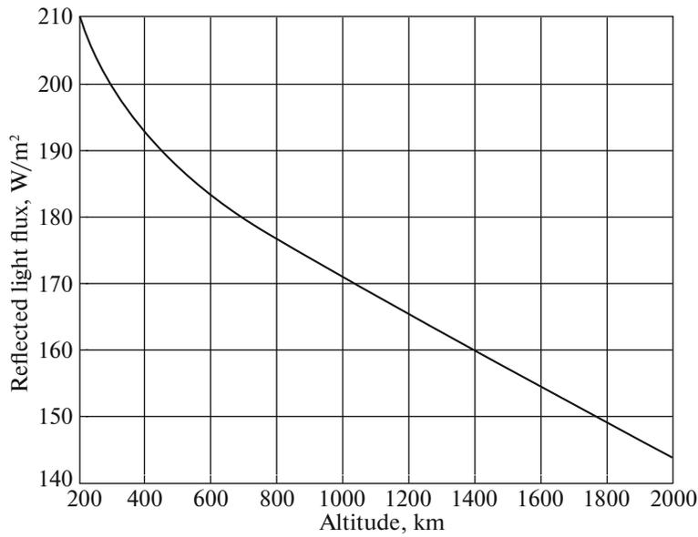
Fig. 2. Earth-reflected solar radiation as function of orbit altitude.
