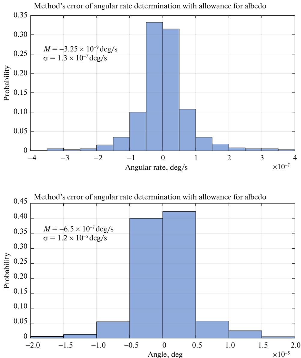
Fig. 7. Distribution of probability of errors of reconstruction of attitude motion parameters with allowance for Earth's albedo.
