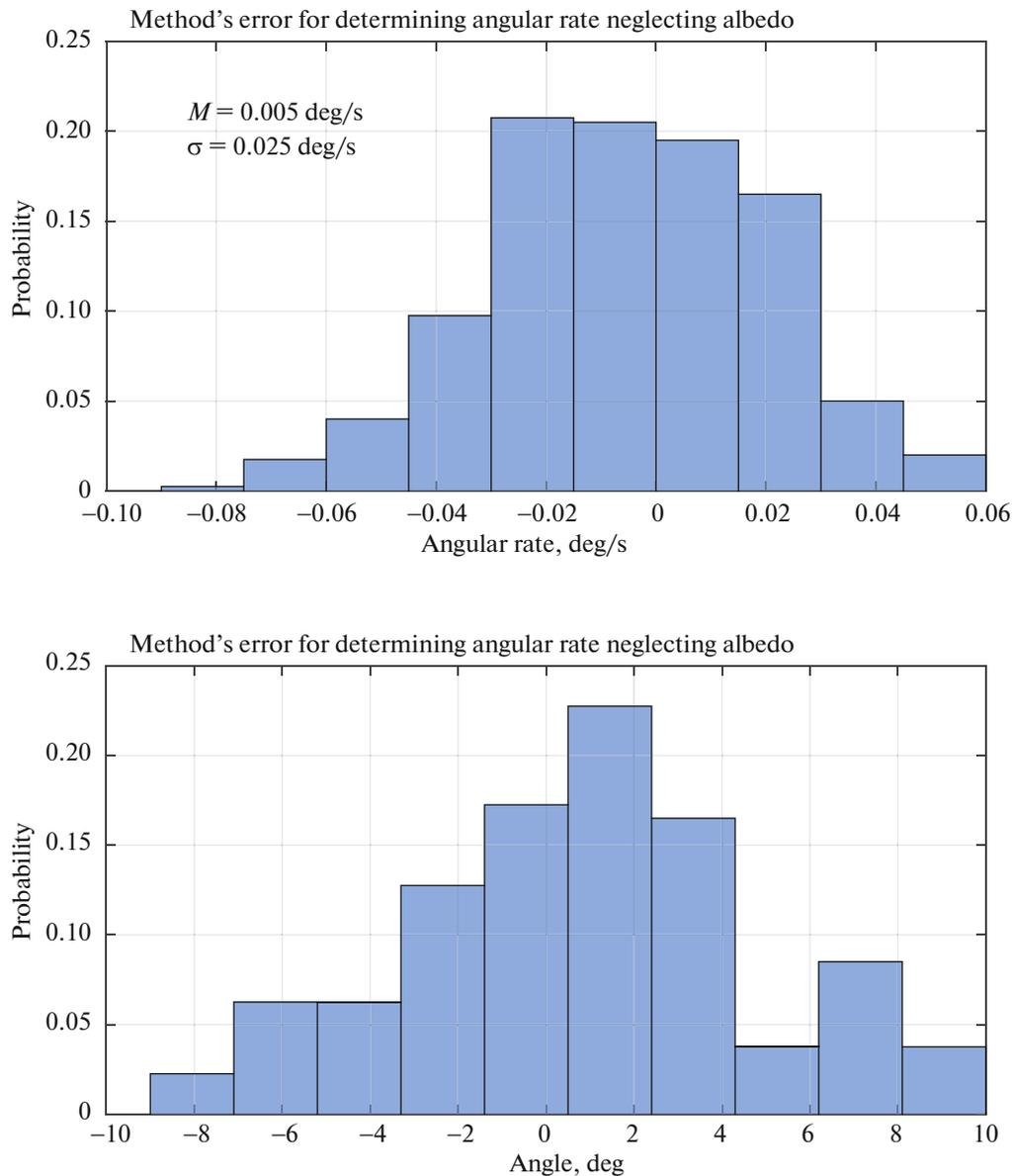
Fig. 8. Distribution of probability of errors of reconstructing attitude motion parameters neglecting Earth's albedo.
